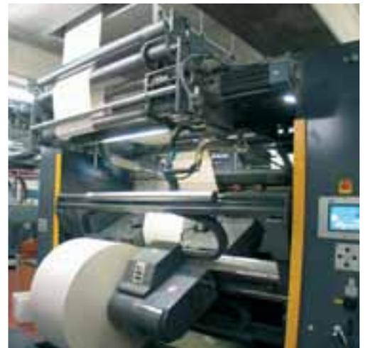
Intelligent Lenze servo inverters, equipped with winder technology functions, can be used for complete reel control, including the reel calculator with precise feedforward control of torque and speed depending on the extent to which the reel is filled.
