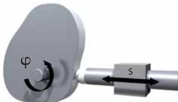
Electronic cam drives imitate cam mechanisms. As many cam characteristics as necessary can be implemented. These provide optimised motion profiles and can be changed in next to no time. The advantages of this are increased flexibility and productivity with modern production and processing machines. The electronic solution reduces the masses to be moved. The advantages of this are increased dynamic performance due to smaller moments of inertia, less wear, smaller drives.
